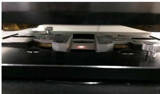
Close up of the Films & Fibers Clamps mounted on the sample holder MicroVice. You can see that a film is fixed with the clamps
