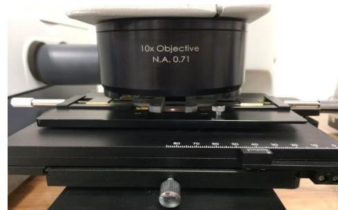
Sample Holder MicroVice with Films& Fibers Clamps set on the microscope stage
