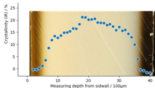
**Step 5.** Spectral analysis of the IR line scans was conducted to derive crystallinity profile. Spatially-resolved quantification of crystallinity via IR band evaluation
