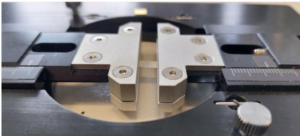
**Step 3.** Setting the MicroVice Holder with the mounted sample onto the stage of the IR microscope
