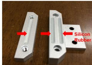
*The upper and lower cylindrical silicone rubbers firmly grip the sample and fix it in place without damaging it.*
