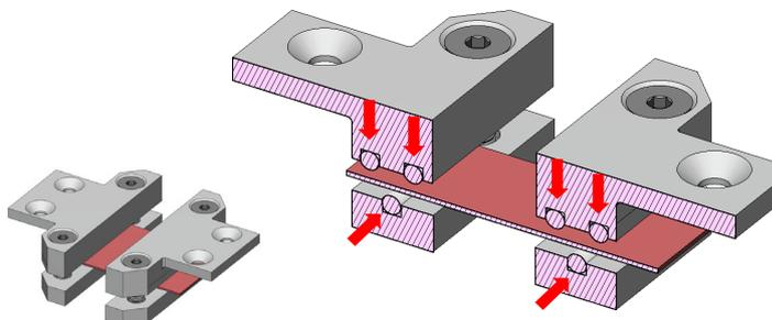
*The design of the clamps ensures that the sample can be fixed flat within the clamps and can be securely and evenly stretched without twisting.*
