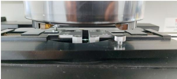
**Step 4.** IR line scans were performed along the cross-section of the microtome cuts
